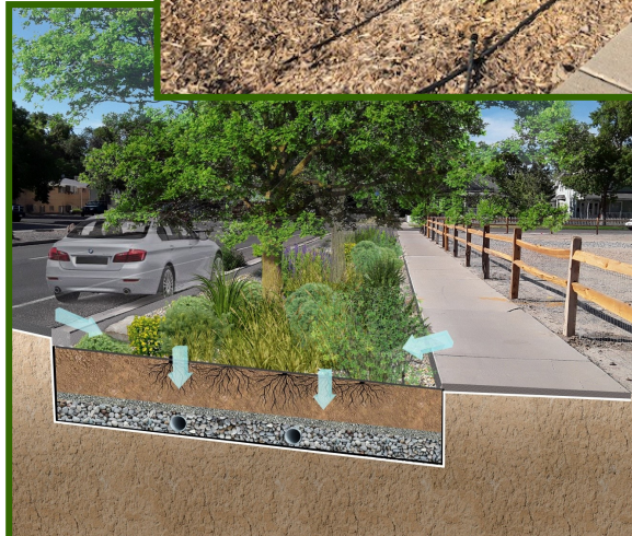
Left: Illustration of cross-cut bioswale construction.
